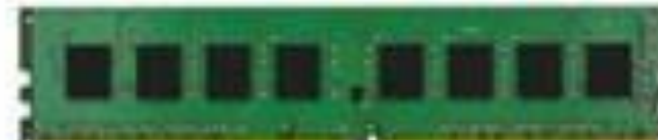
288 pin DDR-4 DIMM note curved edge on pins
